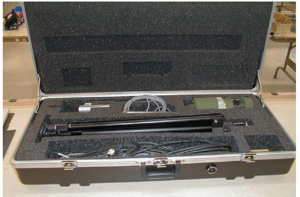
The TACMET II weather station is easily carried in two cases. One case houses the radio, battery and charger, and the other holds the weather station, tripod, mount to attach the sensor to the tripod, and all of the system's cables.
