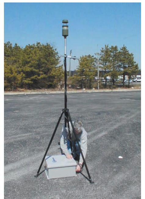
The TACMET II weather station is easily carried in two cases. One case houses the radio, battery and charger, and the other holds the weather station, tripod, mount to attach the sensor to the tripod, and all of the system's cables.
