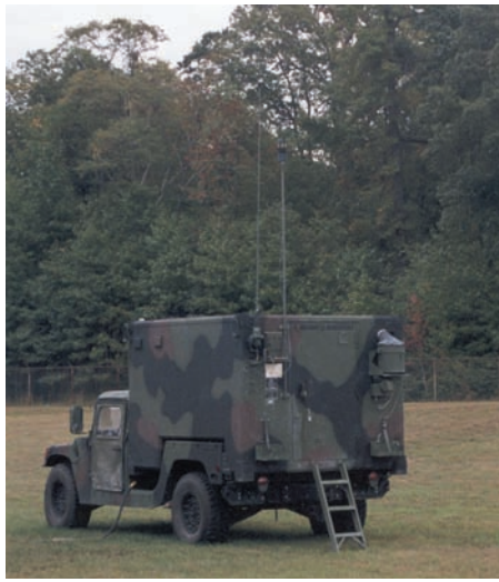
The Biological Identification and Detection System consists of a shelter mounted on a vehicle and equipped with a biological detection suite employing complementary technologies to detect large area biological attacks.
